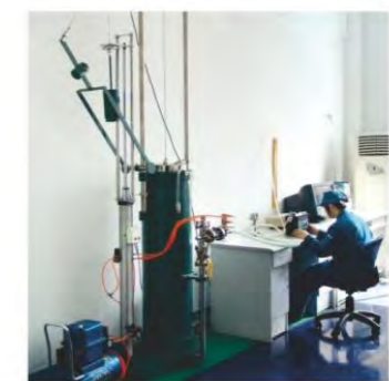
Bell-Prover Gas Flow Standard Device
